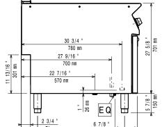
EI = Electrical inlet (power) EQ Equipotential screw Water inlet
